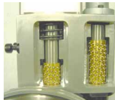
All DF models have ball-bearing knife holder axles
